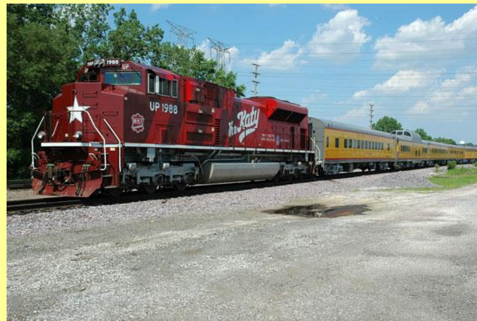
Here's the train at West Chicago. There were units on both ends so it was not necessary to wye the train at Nelson. The E-9 B unit was for head end power.
